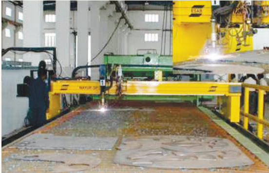
Multitherm ECO CNC plasma profile cutting machine can handle 10 m x 4 m x 50 mm thk
